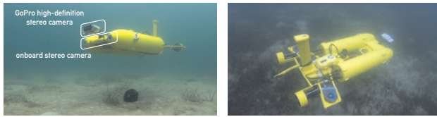
Fig. 8. The Starbug AUV was equipped with an onboard forward looking stereo camera pair. In addition, a GoPro high-definition stereo camera head with 32 mm baseline was mounted to the front of the vehicle and recorded during the experiments.
