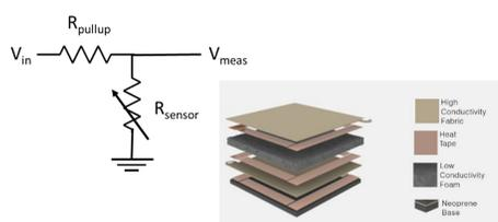
Each sensor covers a segment of NAO's arm and operates as a single tactile.
