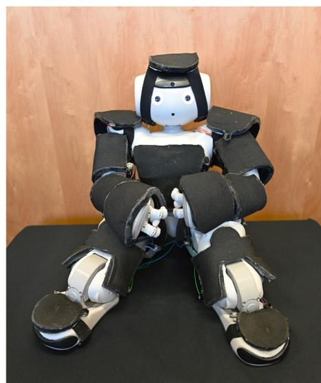
Left: NAO wearing the twelve new sensors we created, along with the original four patterns by Burns et al. Right: The custom receiver and sender components of our microcontroller, which has several hardware upgrades and allows for wireless data transmission.
