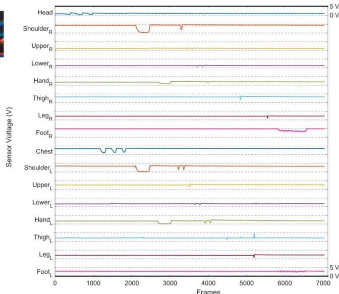
Sample touch interactions measured as time-series voltage data across all 16 channels. The user performs stroking on the robot's head, squeezing its shoulders and hands, poking the arms, hitting the legs, and tickling its feet.
