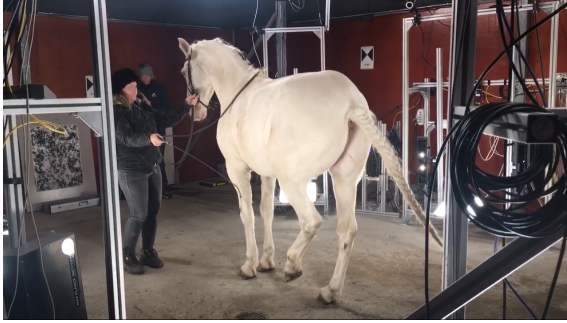
Figure 2. Dynamic 3D horse scanner. The horse is asked to lift one hind limb.
