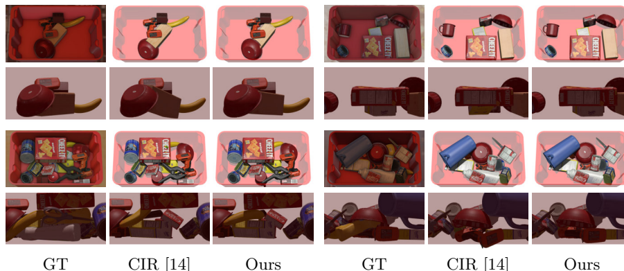
Fig. 3: Qualitative results on the Synpick dataset. Our method manages to reduce penetrations between the objects and the background box, leading to more accurate results for occluded objects (wood block in the top left, sugar box in the top right, banana in the bottom left and power drill in the bottom right). The average AD scores improve from 0.014 to 0.013 (top left), 0.031 to 0.009 (top right) and from 0.031 to 0.023 (bottom right), and remain approximately the same at 0.043 for the bottom left example.
